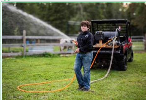
James Johnson Rose Lake Miocene 4-H Club Small Engines Water Pump 2021 BE WP-1020R 1" waterpump, powered by 79cc 4 stroke gas engine
